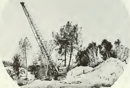
Photo 8. Dragline at American Lignite Products Company, Amador County. The lignite is not produced for fuel, but is used for the making of monton wax. Photo by Mort D. Turner.
