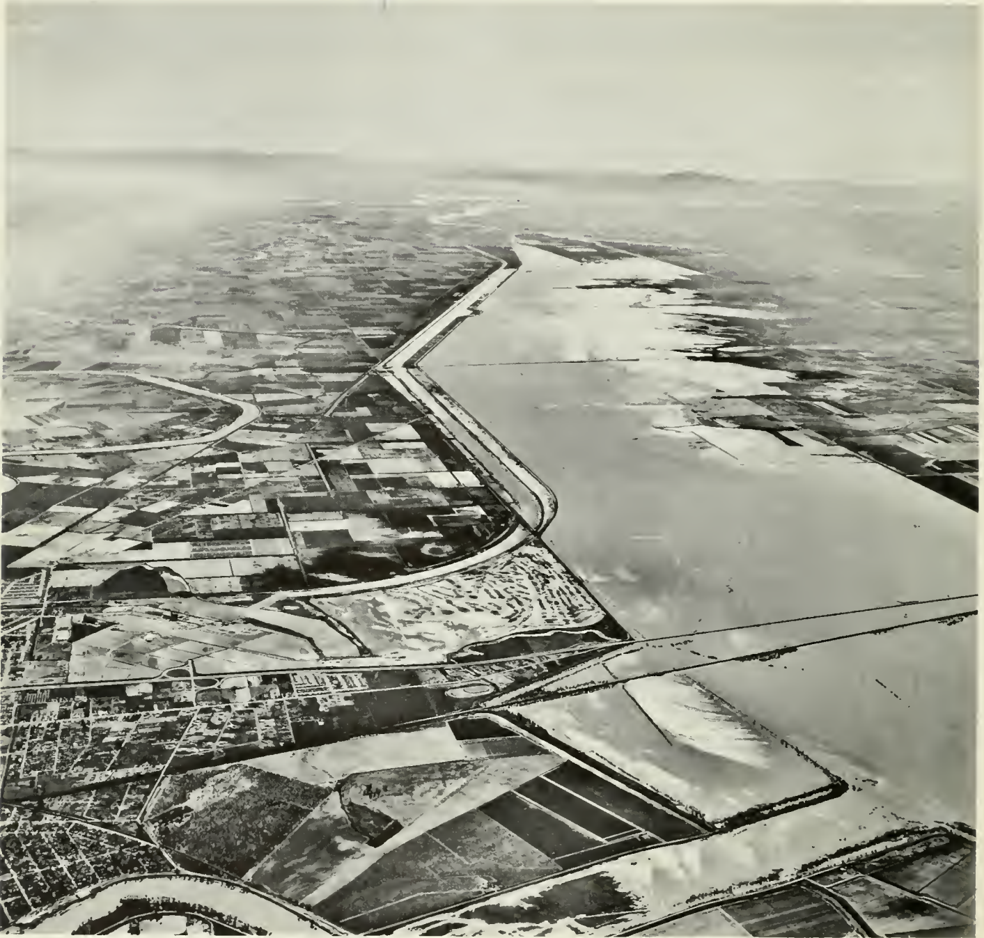
Photo 1. Aerial oblique view of the southern Sacramento basin during high water. The Yolo Bypass, a flood-control waterway, crosses the right middle ground. Mount Diablo is in the right background. Photo courtesy Cartwright Aerial Surveys, Inc., Sacramento.
